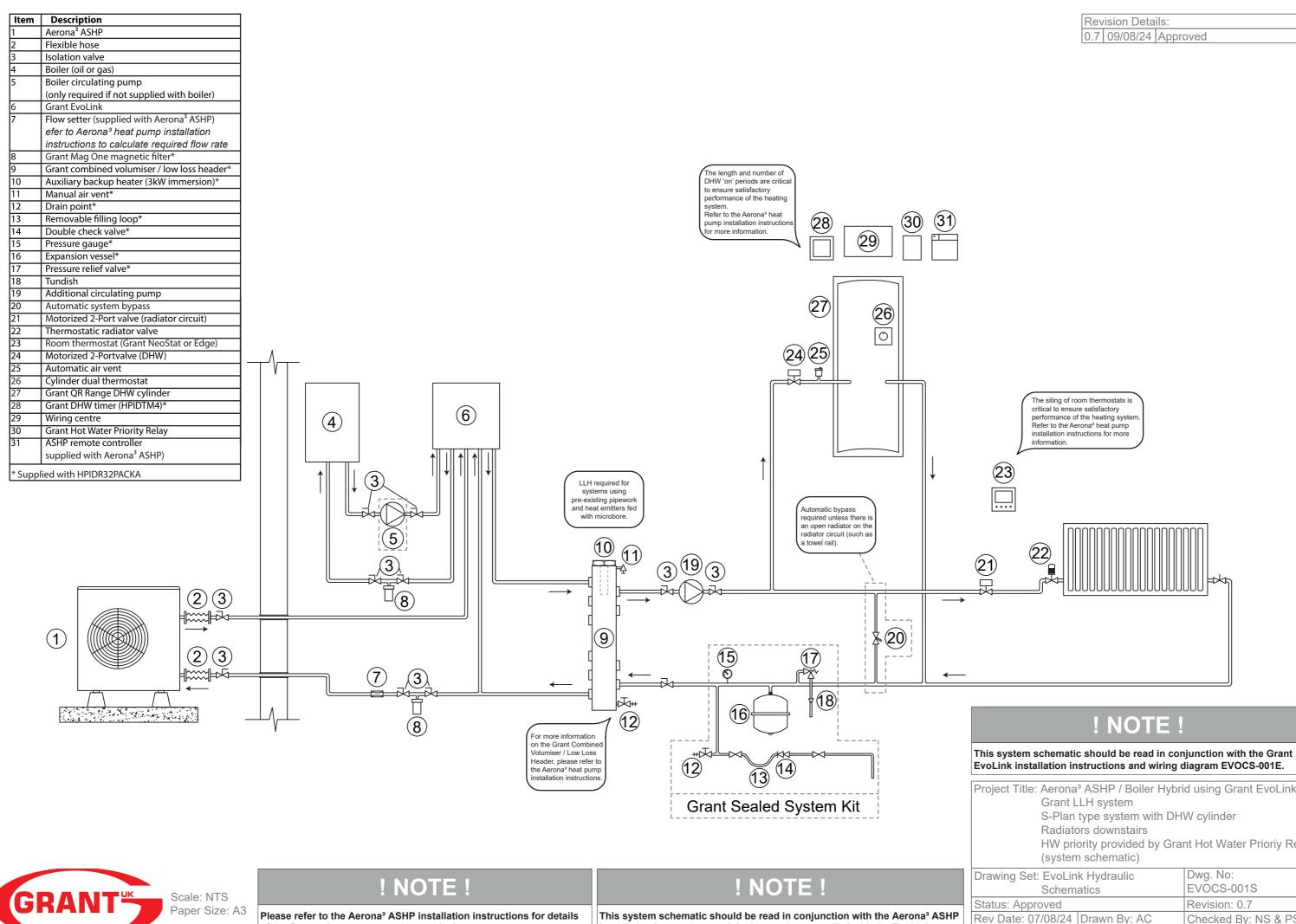
of the flow and return connections at the heat pump.
