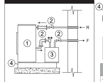
\*\*Compression elbow c/w air vent (supplied with HPIDVOL30EXT6)
