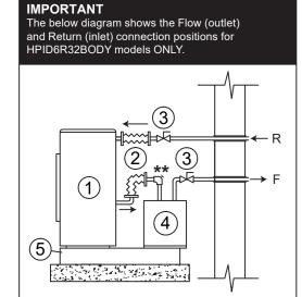
\*\*Compression elbow c/w air vent (supplied with HPIDVOL30EXT6)
