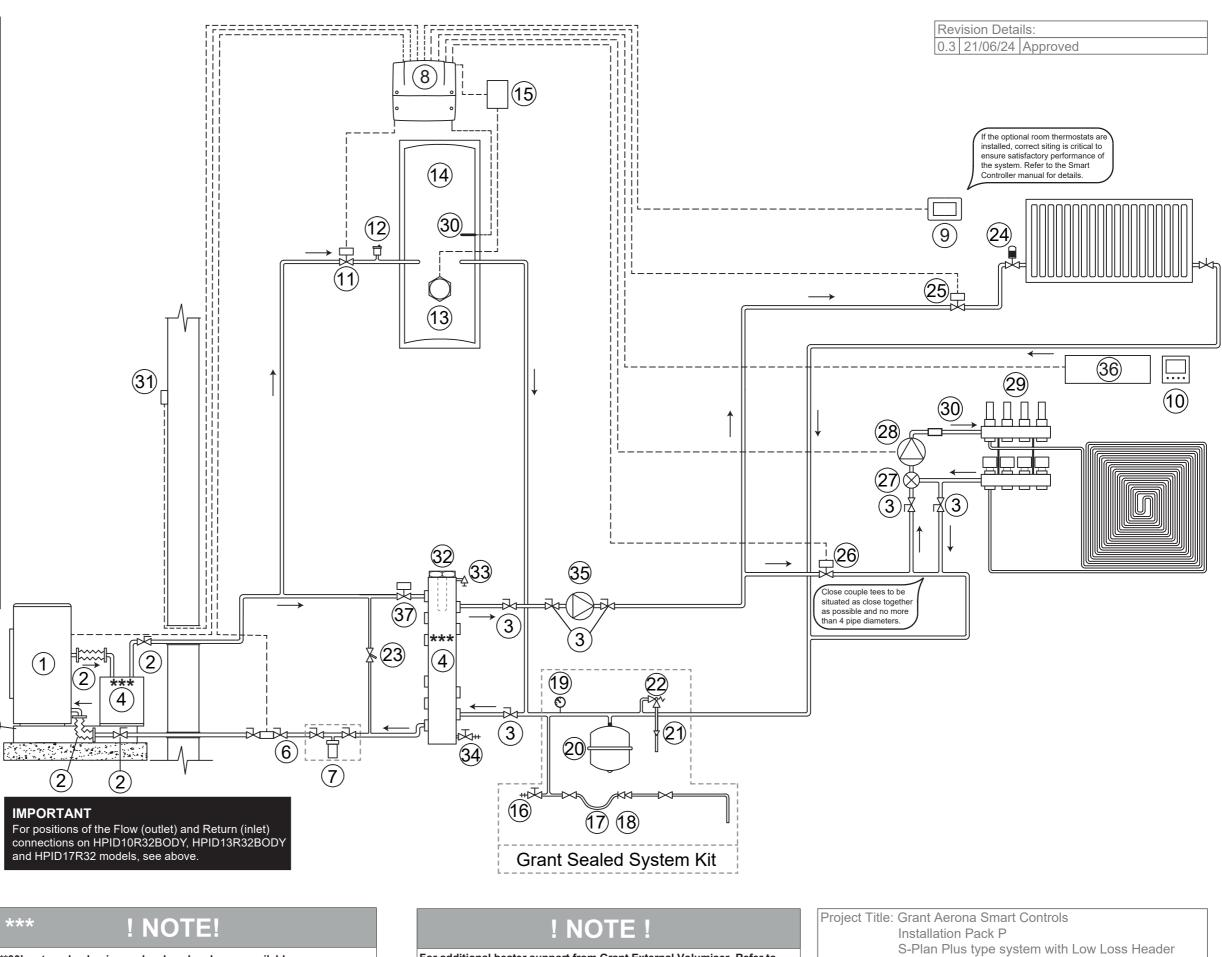
\*\*\*30L external volumiser or low loss header are available as an optional component where there is insufficient system volume or where hydraulic separation is required (HPIDVOLEXT30/HPIDSYSLLHKIT).
