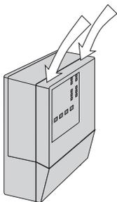
Press down at the fingertip grips on top of the front cover and pull out and down.
