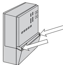
Loosen the screws at the front of the wiring cover.
