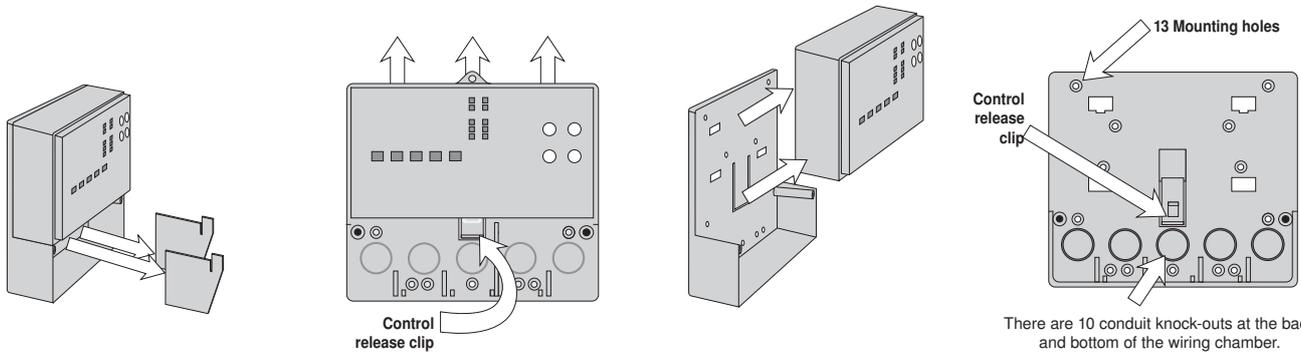
Remove the safety dividers from the wiring chamber by pulling them straight out of their grooves.
