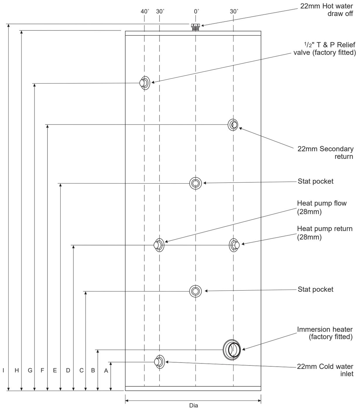
**Figure 2-4:** 'A-rated' MonoWave indirect HP cylinder dimensions
