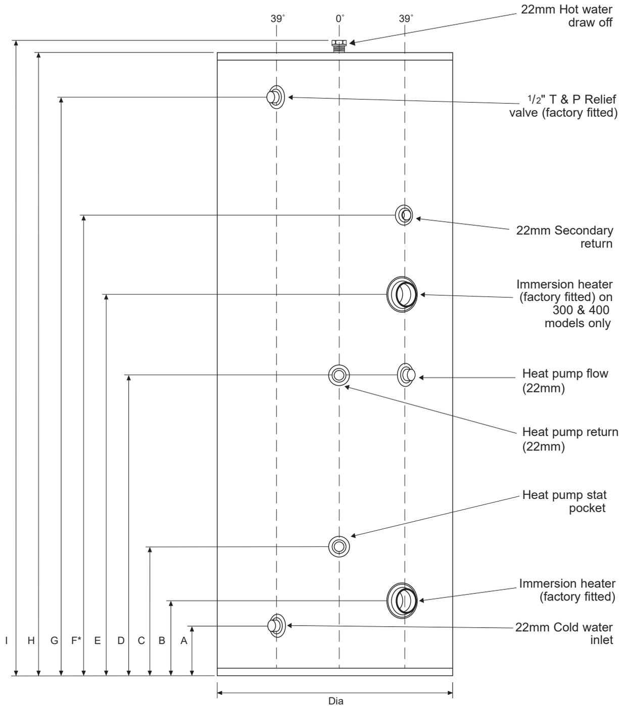
**Figure 2-3:** MonoWave indirect HP cylinder dimensions (excluding 125, 150 and 170L models)
