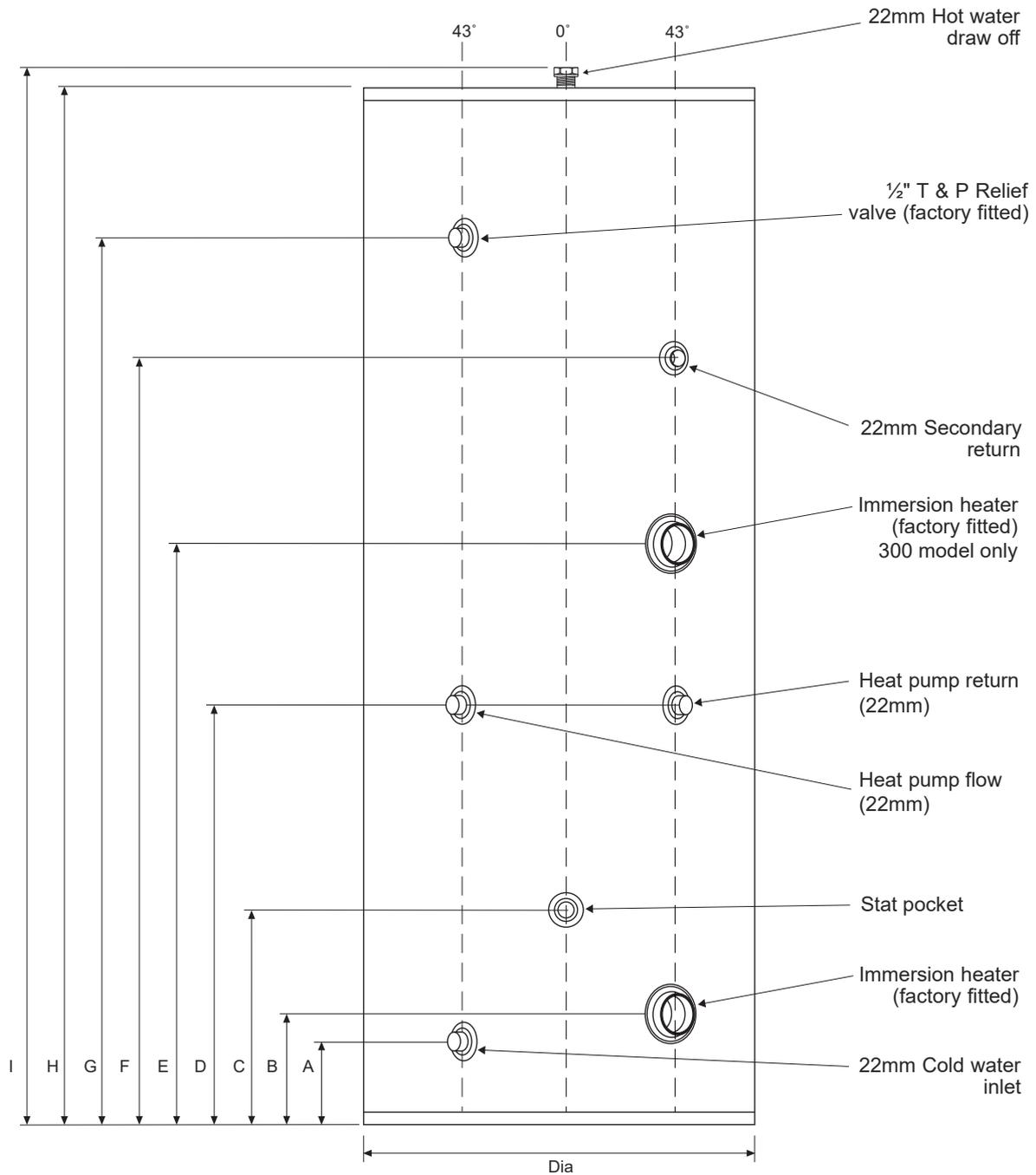
Figure 2-5: Slimline MonoWave indirect HP cylinder dimensions
