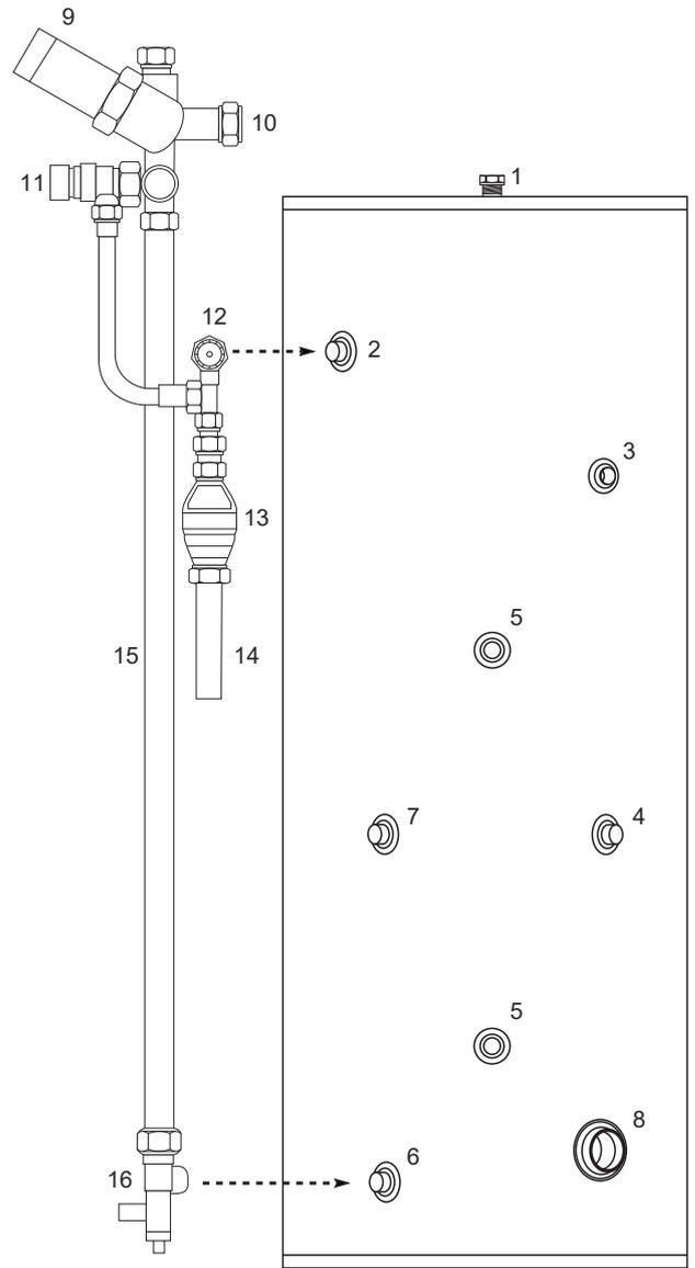
Figure 2-9: 'A-rated' 200L MonoWave indirect HP cylinder
