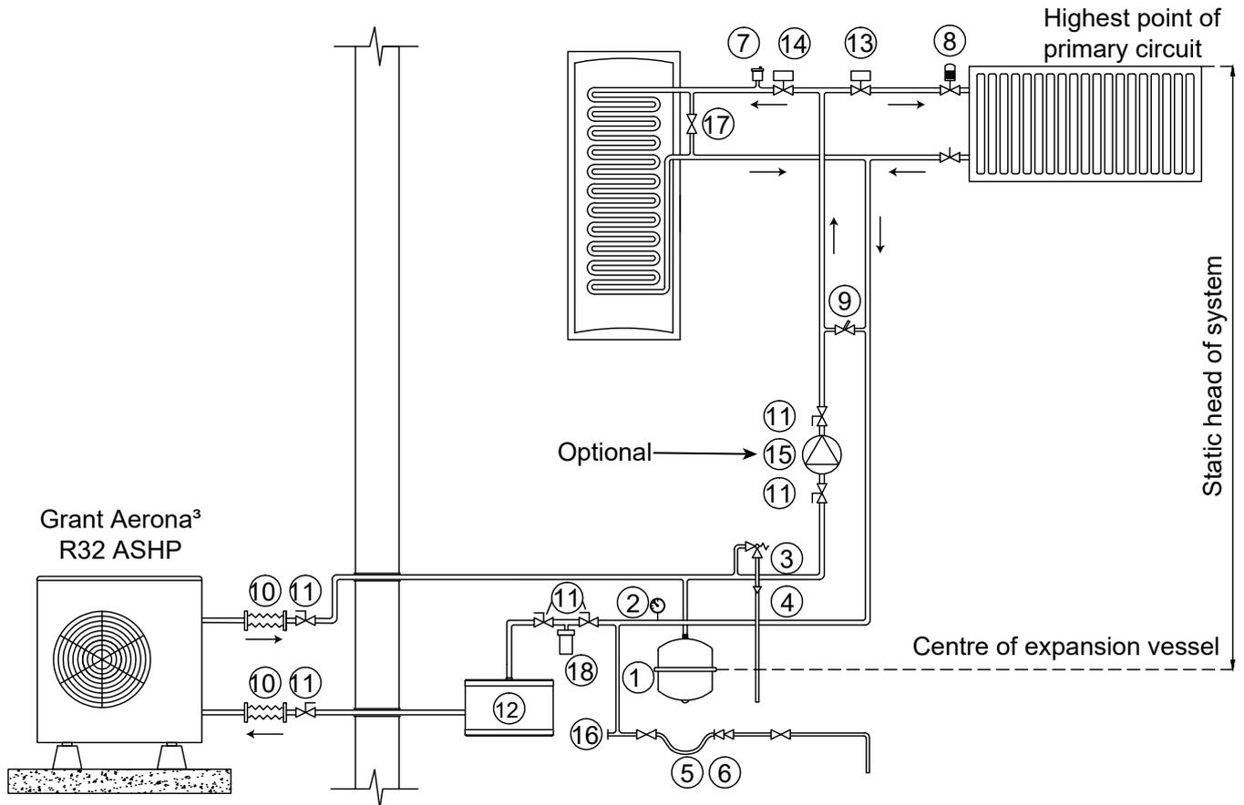
**Figure 5-2:** Monovalent system - with S-Plan type controls
