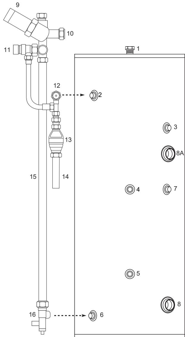
**Figure 2-7:** MonoWave indirect HP cylinders
