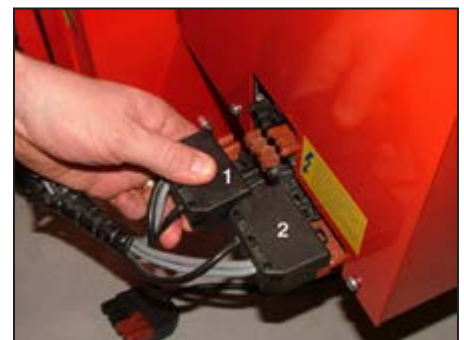
Figure 7-2: Remove plug 1 from burner
