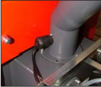
Figure 10-5: Location of thermostat
