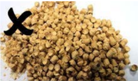
Figure 3-4: Pellets too short in length
