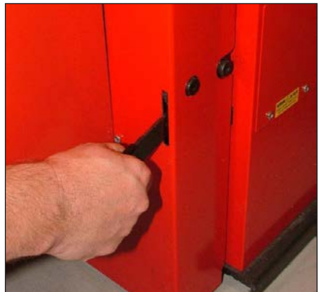
Figure 10-4: Fitting the removable door handle
