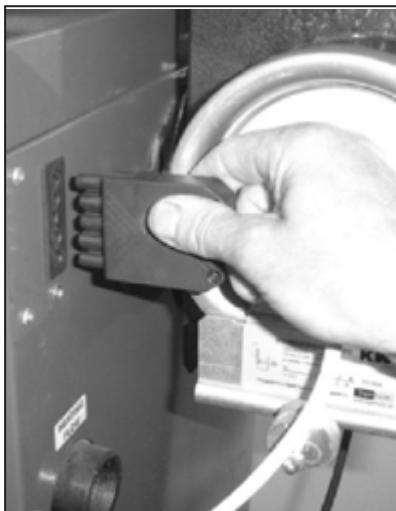
Figure 4-4: Flue fan/solenoid valve plug connection
