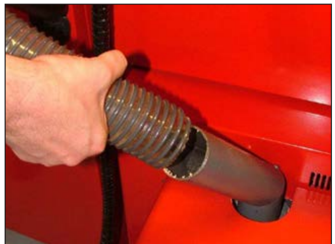
Figure 10-3: Disconnect pellet hose from burner
