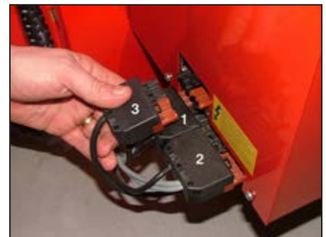
Figure 7-1: Remove plug 3 from burner
