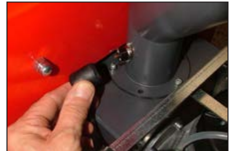
Figure 6-2: Disconnect lead from pellet tube thermostat
