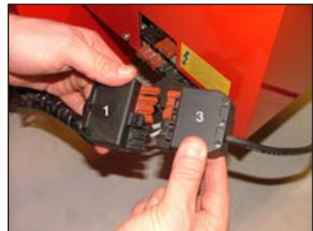
Figure 7-4: Connect plugs together
