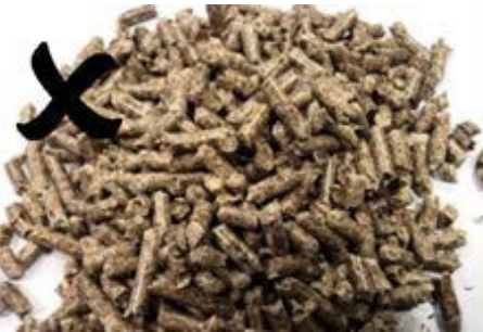
Figure 3-3: Pellets too dark in colour
