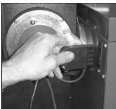
Figure 11-1: Disconnecting hopper 5-way plug
