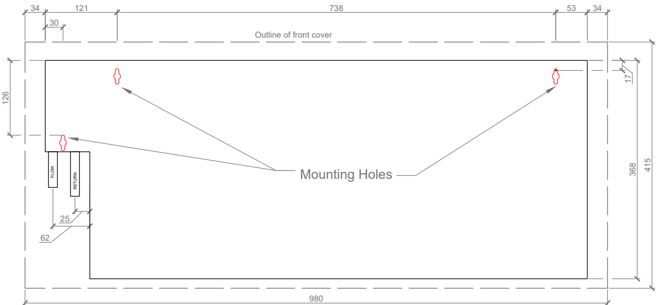
Figure 3-7: Solo CompactMAX fixing holes (viewed from the front)
