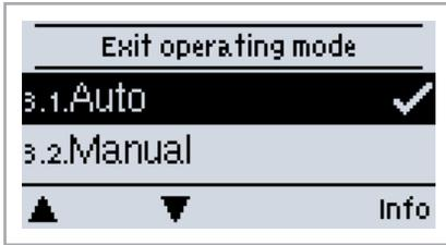
In menu "3. Operating modes" the controller can either be placed in automatic mode, switched off, or placed in a manual operating mode.
