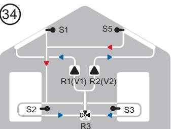
Solar with 2 collector surfaces, 2 storages and 2 pumps
