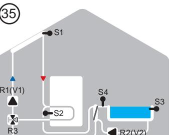
Solar with swimming pool, storage, heat exchanger and valve
