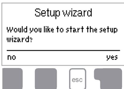
The first time the controller is turned on and after the language and time are set, a query appears as to whether you want to parametrise the controller using the commissioning help or not. The commissioning help can also be terminated or called up again at any time in the special functions menu. The commissioning help guides you through the necessary basic settings in the correct order, and provides brief descriptions of each parameter in the display.
