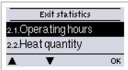
The menu "2. Statistics" is used for function control and long-term monitoring of the system.
