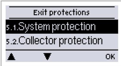
Menu „5. - Protections / Protective functions“ can be used to activate and set various protective functions.
