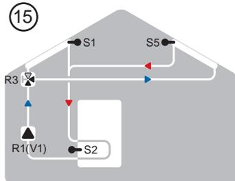
Solar with 2 collector surfaces and switching valve
