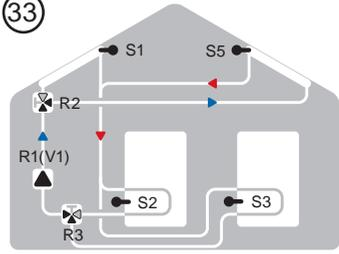
Solar with 2 collector surfaces, 2 storages and 2 valves
