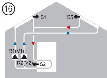
Solar with 2 collector surfaces and 2 pumps
