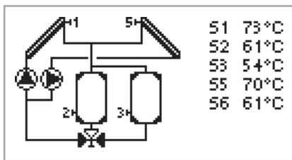
The graphics or overview mode appears when no key has been pressed for 2 minutes, or when the main menu is exited by pressing “esc”.
